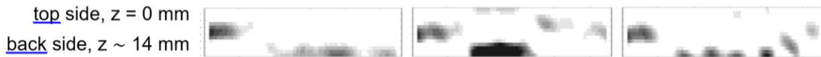
Figure 5: Scan results displayed as B-scans, not to scale. From left to right: coordinate y near to top edge, medium, and near to bottom edge of fig. 4.
