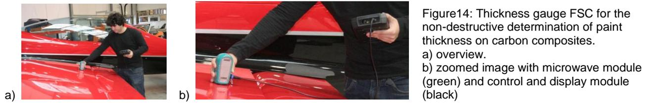
Figure14: Thickness gauge FSC for the non-destructive determination of paint thickness on carbon composites.
