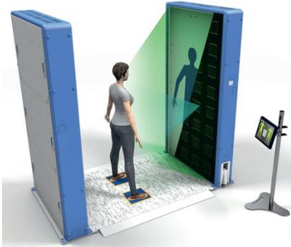
Figure.10: The body scanner R&SR<sup>®</sup>PS uses frequencies between 70 GHz and 80 GHz with a radiation power of 1 mW and each 3008 transmit and receive antennas. One after the other the antennas and 128 frequency channels are activated. This leads to a scan time as low as 32 ms.
