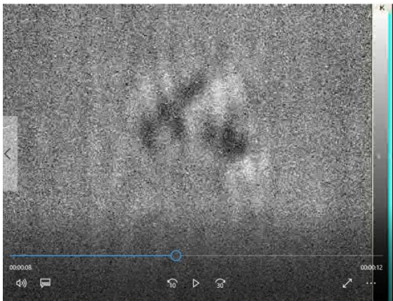
Figure 4: NIDIT image of the plane plank 2 in the region of the crack.
