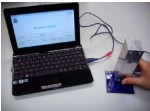
Figure 1: Paint thickness gage FSC1 consisting of the measuring module and the display module.
