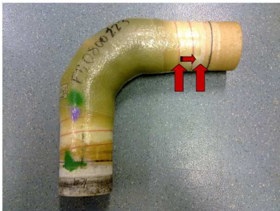
Figure 4: Elbow from GFRP with sand, wall thickness about 5 mm
