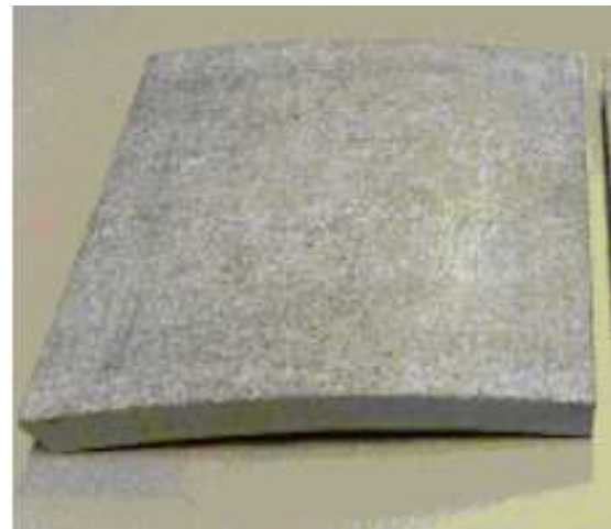
Figure 1. Bended Plate with dimensions 200 mm x 200 mm x 22 mm.
