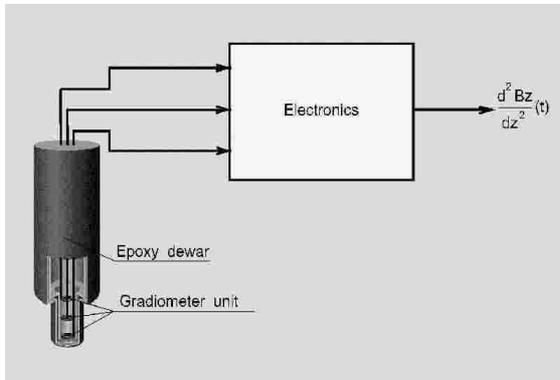
Fig. 2: Principle view of second-order gradiometer
