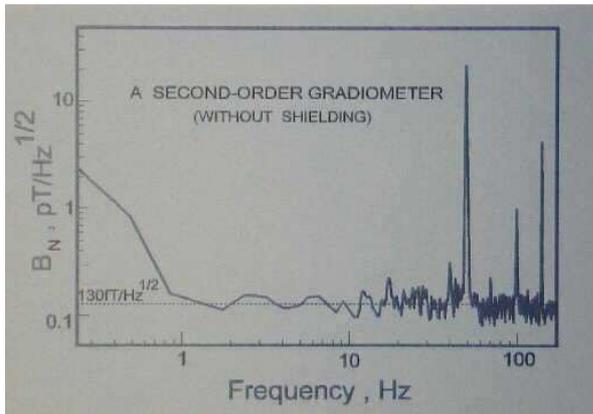
*Fig. 3: Magnetic field noise  $B_N$  of HMT Magnetometer System*
