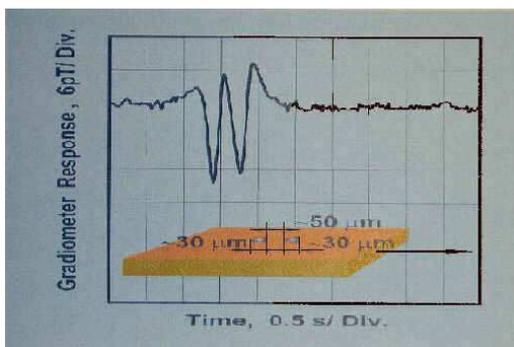
*Fig. 6: Gradiometer response measured during the motion of two ferromagnetic particles in real time. The insert represents a schematic view of the experimental setup of both particles*
