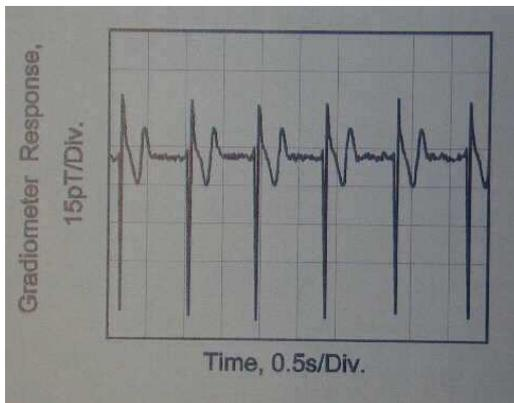
*Fig.5: Human heart signal (Magnetocardiogram) measured without magnetic shielding*
