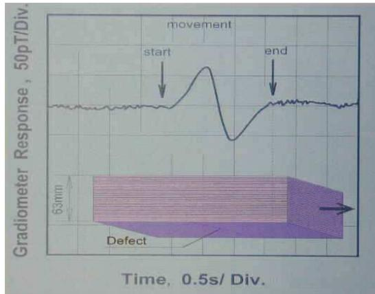
*Fig.7: Detection of hidden cracks below layers of aluminium plates*
