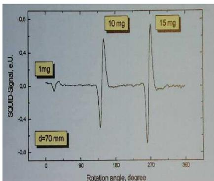
*Fig.4: SQUID-Signals of Defects with Different Masses*
