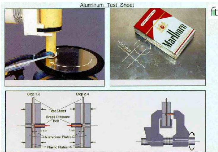
Fig. 1: Creating plastic deformation in the aluminum test sheet.
