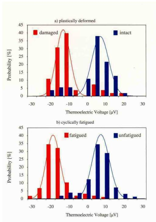
Fig. 3: Probability of thermoelectric voltage measured with a contacting method on Ti-6Al-4V bars. a) plastically deformed and b) cyclically fatigued sample, both compared with untreated samples.
