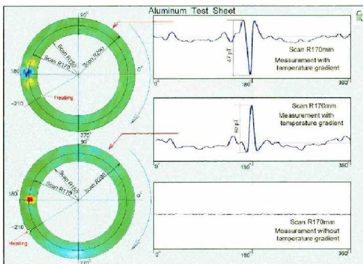
Fig. 2: Measuring results using the Thermoelectric SQUID Method.
