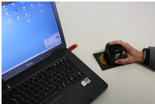
Figure 1: Paint thickness measurement system, consisting of measurement module and display module (here laptop)
