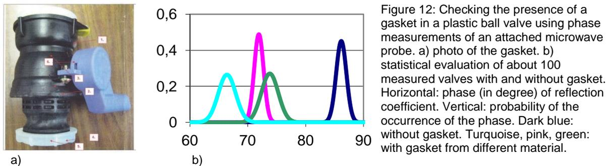
Figure 12: Checking the presence of a gasket in a plastic ball valve using phase measurements of an attached microwave probe. a) photo of the gasket. b) statistical evaluation of about 100 measured valves with and without gasket. Horizontal: phase (in degree) of reflection coefficient. Vertical: probability of the occurrence of the phase. Dark blue: without gasket. Turquoise, pink, green: with gasket from different material.
