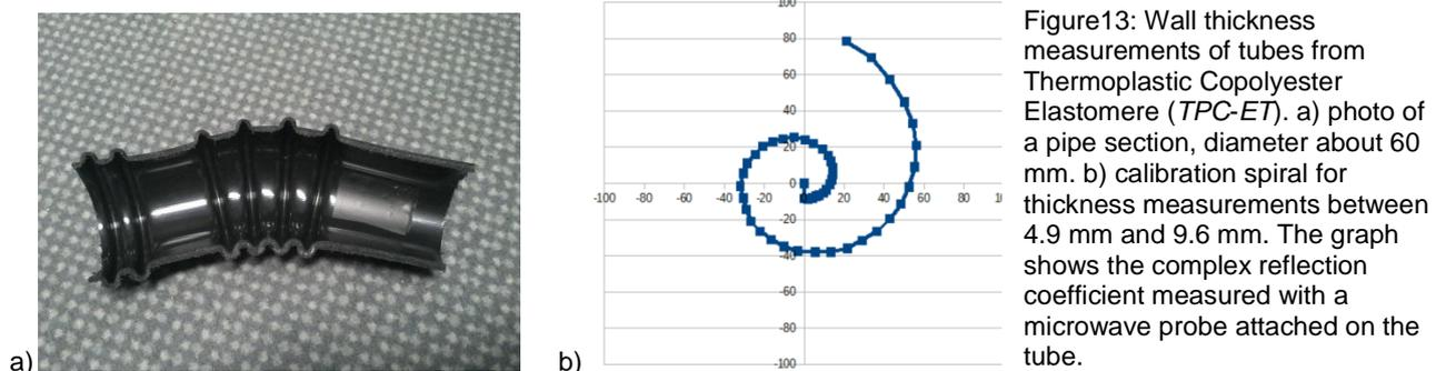
Figure13: Wall thickness measurements of tubes from Thermoplastic Copolyester Elastomere (TPC-ET). a) photo of a pipe section, diameter about 60 mm. b) calibration spiral for thickness measurements between 4.9 mm and 9.6 mm. The graph shows the complex reflection coefficient measured with a microwave probe attached on the tube.
