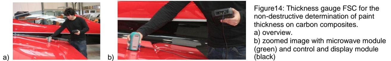
Fig. 14 shows the FSC, in use for paint thickness measurement on a CFRP aerobatic aircraft. Meanwhile the instrument is in regular use in the manufacturing and maintenance processes of widebody and further aircrafts.
