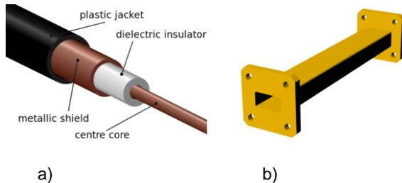
Figure 4: Typical transmission lines for microwaves
