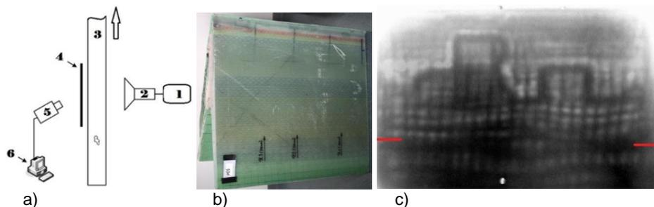
Figure 11: The direct imaging NIDIT procedure: a) principle view, b) sample DUT: cutout of the trailing edge of a rotor blade, c) single video frame of b) with distribution of adhesive
