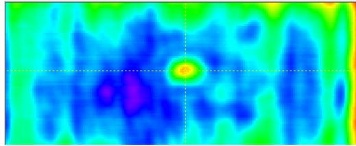
Figure 7: Wall of GFRP pipe. C-scan of a flaw in a depth of 60 mm, 24 GHz
