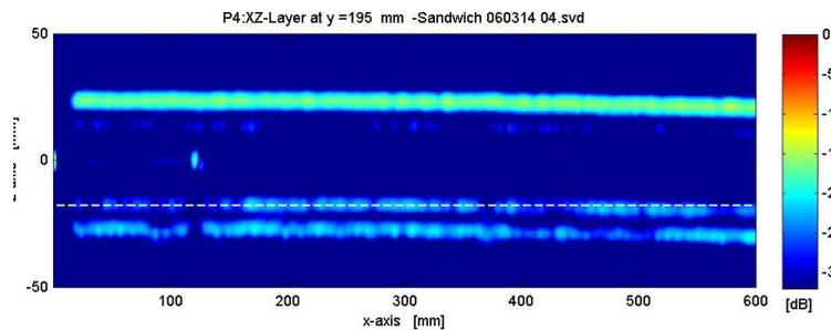
Figure 8: B-scan of a foam/GFRP sandwich at 100 GHz. The indication at 120 mm results from moisture at the interface between foam and GFRP in a depth of about 35 mm. (Becker, Keil: Jahrestagung DGZfP 2017, paper Mi3C2)
