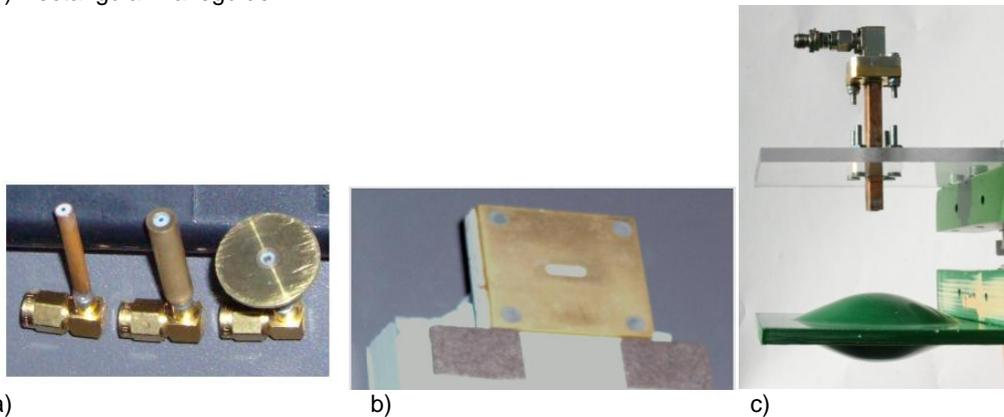
Figure 5: Microwave probes. a) Coaxial antenna. b) Waveguide antenna with iris. c) Lens antenna with open ended rectangular waveguide as primary radiator.
