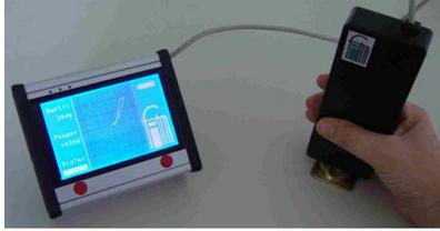
Figure 6: Hand-held microwave NDT instrument
