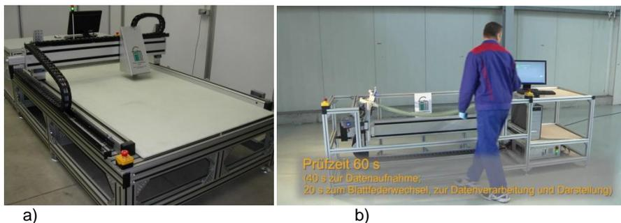
Figure 9: Stationary microwave test systems for a) planar substrates, b) GFRP leaf springs for automobiles.
