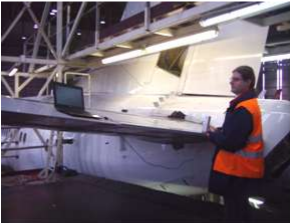
Figure 3: Measuring the paint thickness on the left elevator
