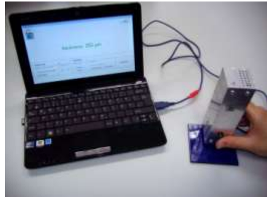
Figure 1: Paint thickness gauge FSC1 consisting of the measuring module and the display module.
