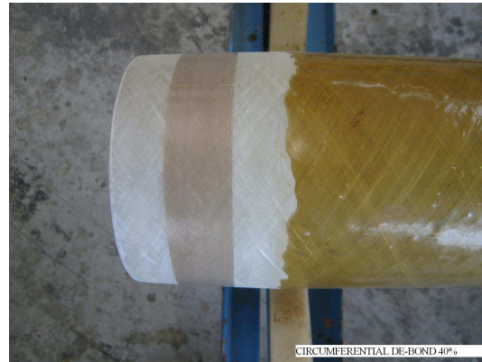
Figure 2: Photograph of one pipe end with artificial debond
