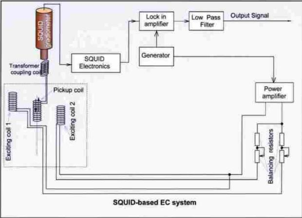
Figure 3 . Block diagram of SQUID-based EC system (please click on image to enlarge).
