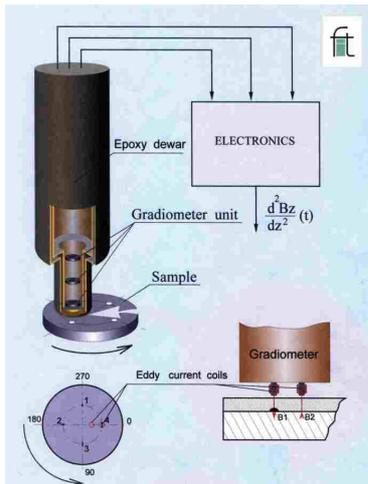
Figure 1. Principal view of the measurement system (please click on image to enlarge)
