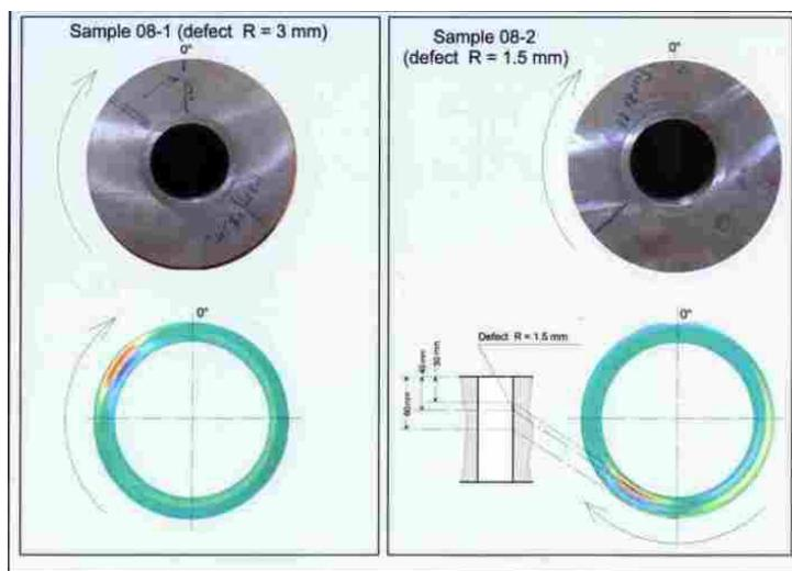
Figure 8. C-Scan diagrams of sample with artificial defects inspected with the LFEC technique. Spacing is 5 mm. Left: defect radius 3 mm. Right: defect radius is 1.5 mm (*please click on image to enlarge*).
