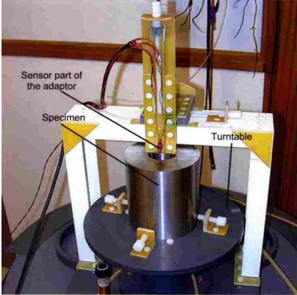
Figure 4. Photograph of a specimen and the sensor part of the adaptor (please click on image to enlarge).
