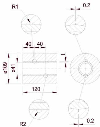
Figure 5. Drawing of the samples with artificial defects (*please click on image to enlarge*).
