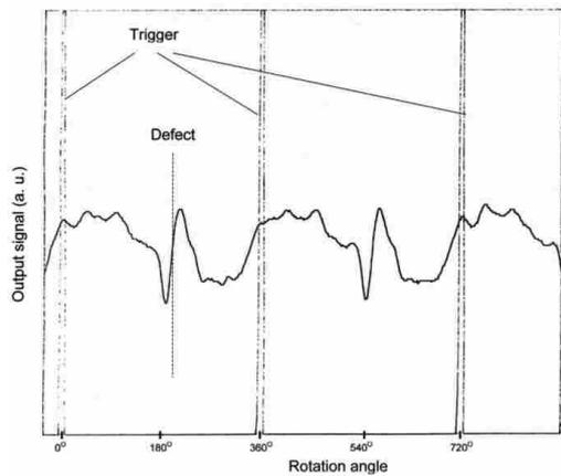
Figure 7. Output signal versus rotation angle for a defect of radius 1.5 mm and 5 mm below the surface (*please click on image to enlarge*).
