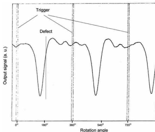
Figure 6. Output signal versus rotation angle for a defect of radius 0.35 mm lying 1 mm below the surface (*please click on image to enlarge*).
