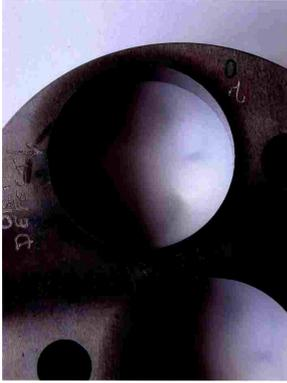
Figure 9. Sample with bore hole #2 and natural defect. The angular position of the defect is marked by an arrow (*please click on image to enlarge*).
